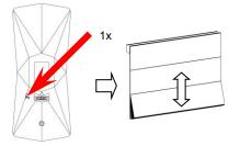
adjust desired lower end limit and press P2 to save the lower limit
