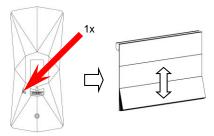
press OPEN button on remote, motor will jog to acknowledge:
